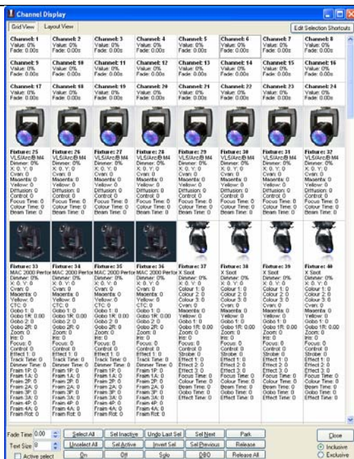
Figure 33: A channel window with 16 moving lights patched from dimmer 25 onward.
